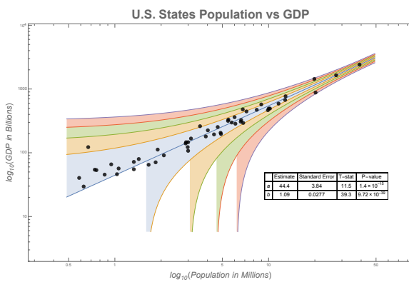
Figure 1. (Left) The figure (Source: [16]) shows the predicted power function line in log-log coordinates (blue line), the data points (as black dots), the sigma bands of confidence (in alternating colors beginning around the predicted power function), and the ANOVA table (on the bottom right).
